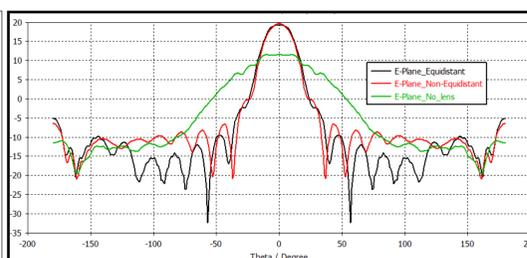
The graph above displays the farfield curves of the E-Plane for the three cases; Non-equidistant lens (red), Equidistant lens (black) and the pyramidal horn antenna in single mode (green).
