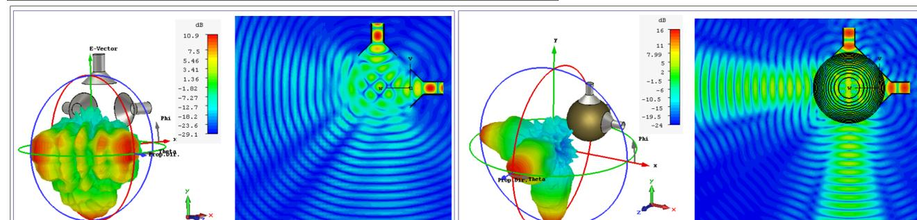
A graphical view indicates the propagation pattern of Luneburg lens when it's fed by multi-feeding conical horn antennas (right) in comparison to the case without the lens (left). With a view of the farfield in both cases.
