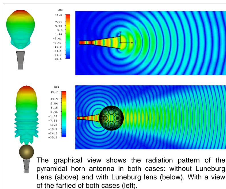
The graphical view shows the radiation pattern of the pyramidal horn antenna in both cases: without Luneburg Lens (above) and with Luneburg lens (below). With a view of the farfield of both cases (left).
