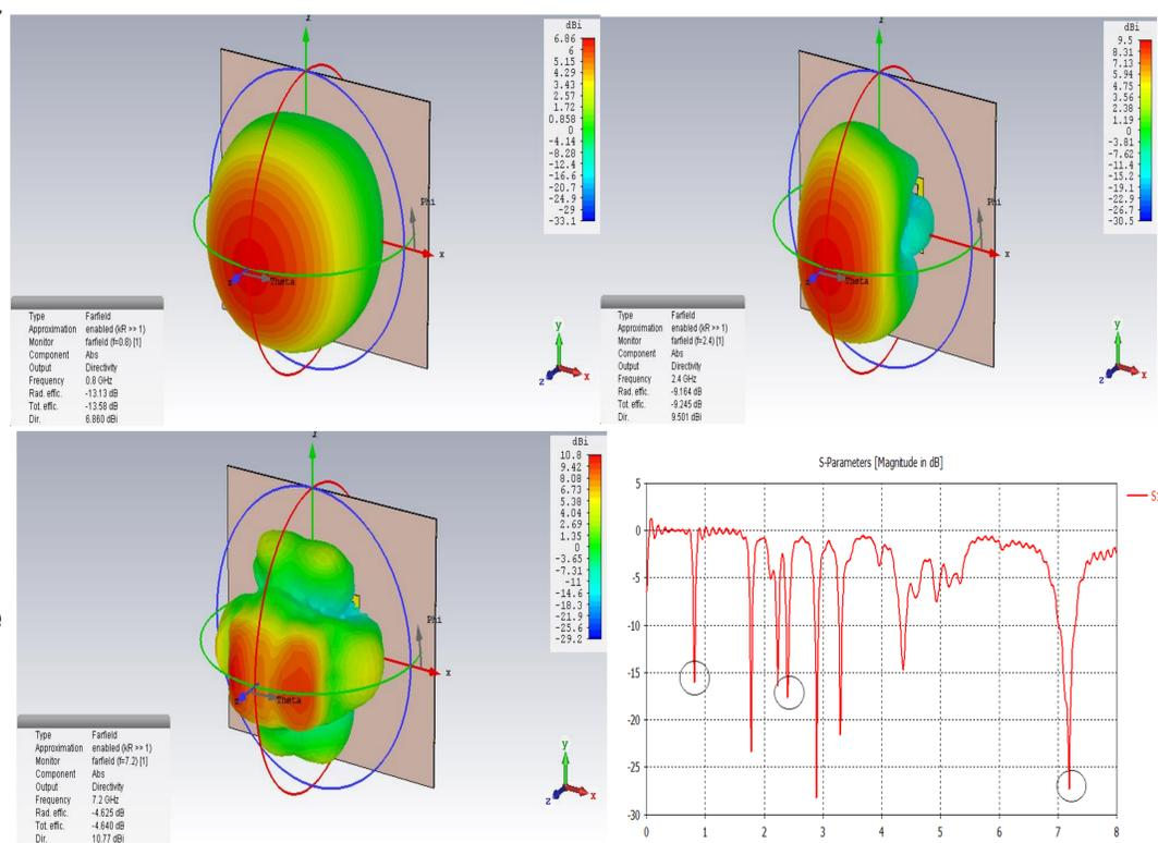
Figure 3: S11 parameters and 3D far field plots of the radiation pattern of a coaxially fed Sierpinski carpet at 0.8GHz, 2.4GHz, and 7.2GHz in its second iteration state
