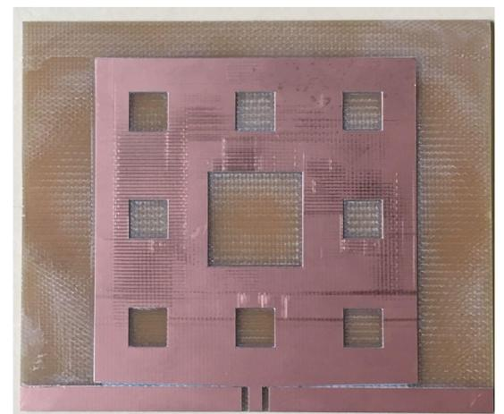
Figure 2: A manufactured Sierpinski carpet to the 2nd iteration with coplanar waveguide feeding method
