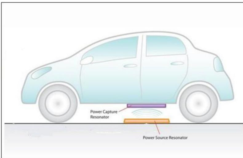
Figure 1 Electric Car with the Power capture and source resonators
