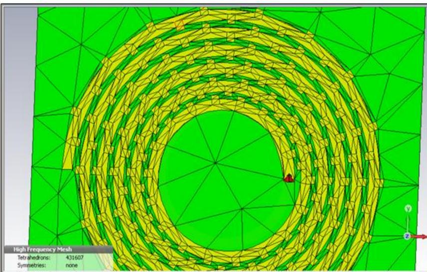
Figure 3 Spiral with inserted stubs, without Boolean add (Mesh View)
